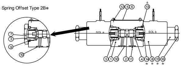
Solenoid assembly is composed of the parts marked with ★.
